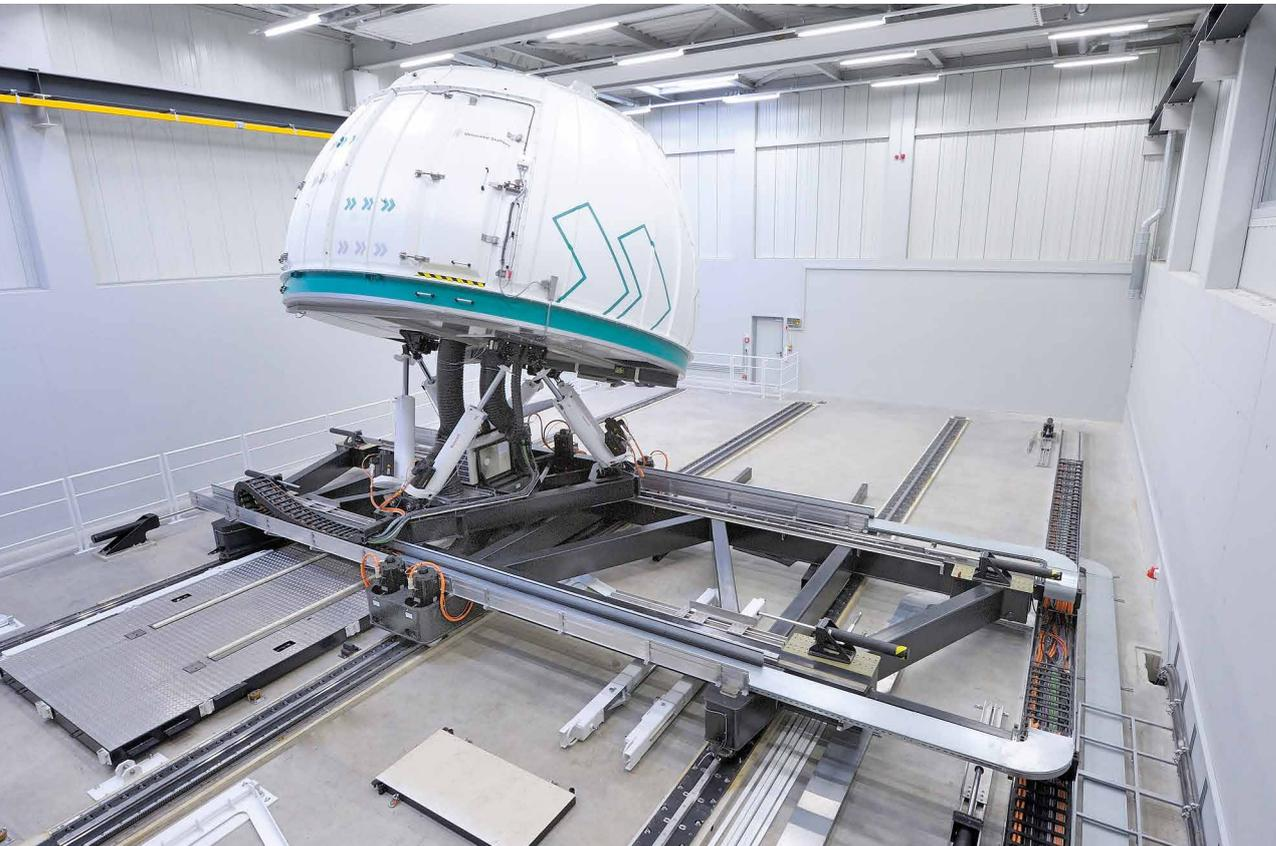
High-performance dampers enable controlled, safe operation of a driving simulator all the way to its end positions.
